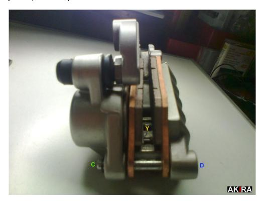
Finally also disassemble the two plates X and Y in steel, clean and grease them, as the sliding pin K.
