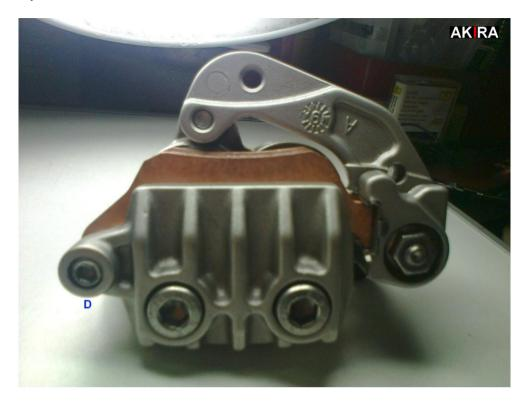
At this point, remove the tablet from the right, then push the left one on the stop to retract the pistons, and then pull
